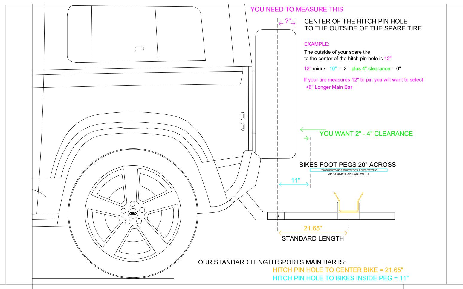
RACK N RIDE HITCH MOUNTED MOTORCYCLE CARRIER SPORTS MAIN BAR STANDARD DIMENSIONS
